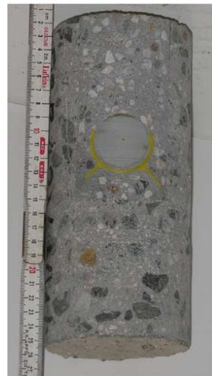
**Figure 2.33. Core DBR42NNW with FRP dowel located 23 mm above mid-depth of slab.**
